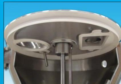
Traditionally, four clamps secure the hopper seal by pulling the hopper up against the hopper cover. The new design has a more efficient lateral-force seal. When the hopper door swings into place, the horizontal pressure from the clamps ensures an airtight hopper seal.
