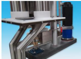
**Do you need a competitively priced filler for your dry food, beverage, pharmaceutical or chemical application?** The Revolution powder filler delivers fast fills with less maintenance thanks to its servo motor auger control and direct drive design. You get a full-color touch screen operator interface, PLC based controls and non-proprietary electrical components. It supports a 5g to 5 lb. fill range and reaches up to 120 fills/minute.
